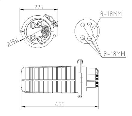
Cable hole can be customized, 3-5mm or 8-18mm
